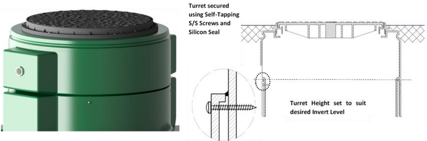
Figure 8: Reduced Turret Height Image and Modifying the Tank Invert Level (NOT applicable to HC6/HC8 models )
